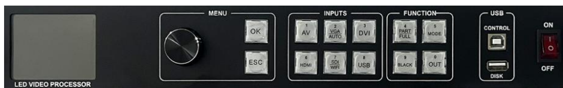
Figure 3—Video Controller front panel
